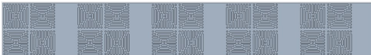
Figure 6: CREO Parametric model of the interfacing side of the device. The four-quadrant pattern alternates between two resisting orientations and has space to accommodate vascular channels.
